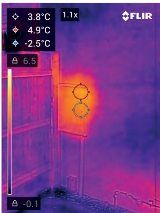
Figure 10 shows thermal images of the outside of a home, the brighter areas showing where additional insulation would reduce heat loss.
